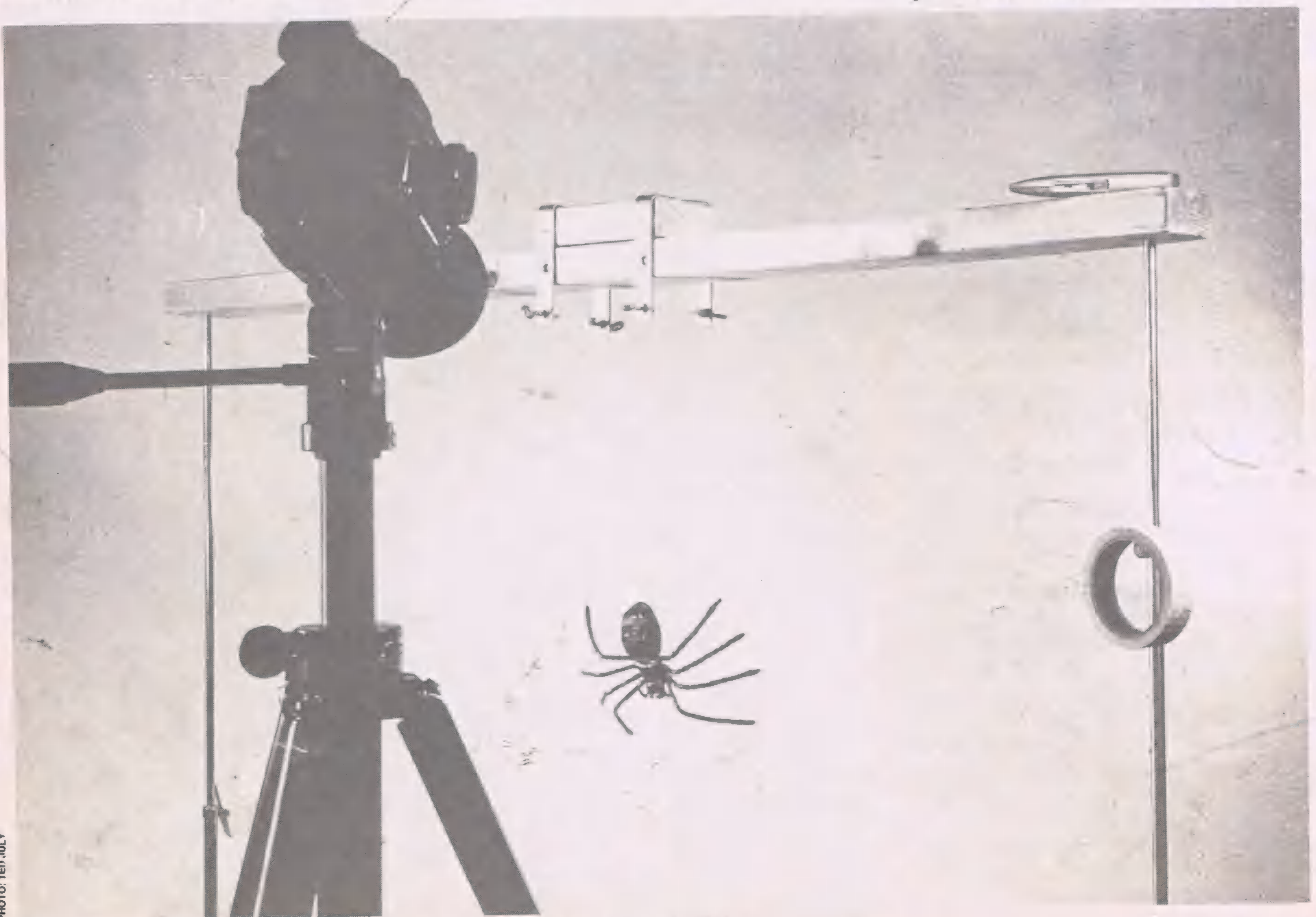
The completed Simplified Aerial Brace rigged with suspended spider creature ready for filming.
